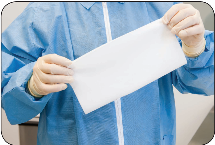
(5) Wiper may be completely unfolded, reversed, and refolded beginning again at Step 1 to enclose the four contaminated faces and expose the four remaining clean faces.
