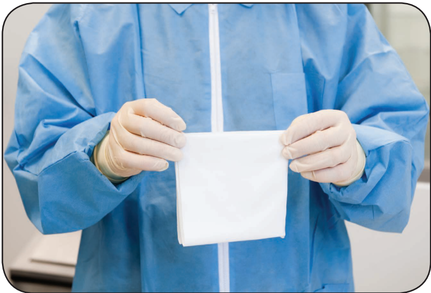
(2) Fold the wiper in half again, creating four cleaning faces: two outside and two inside
