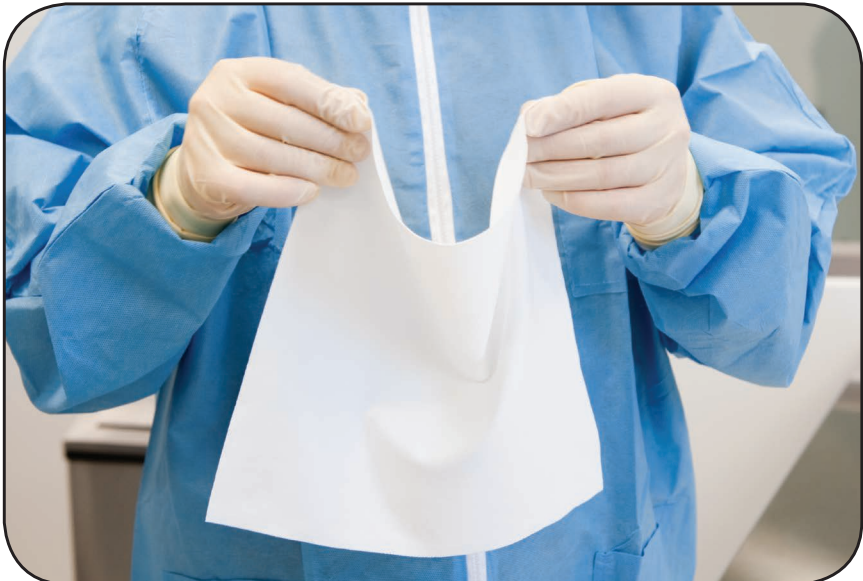
(1) Hold the wiper in mid-air. Take the wiper by its edges and fold in half. The wiper should not be placed on any surface during the folding action.
